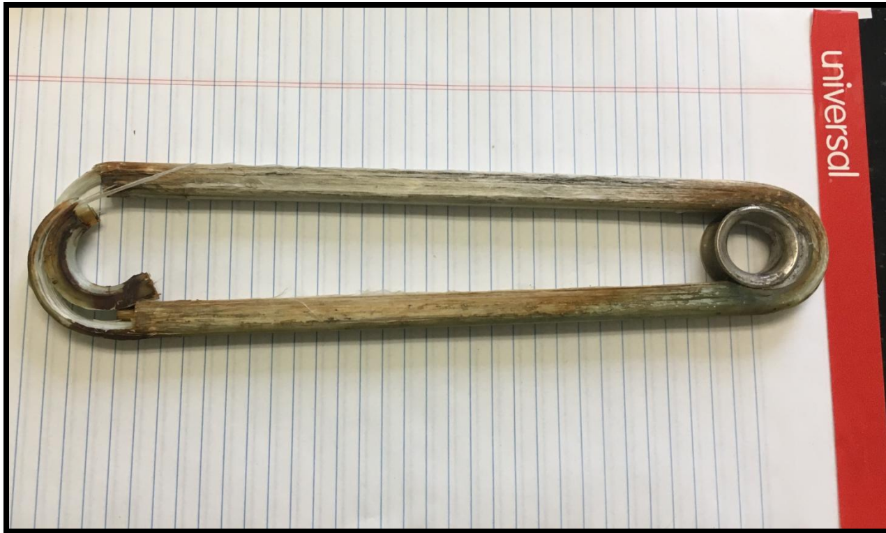
Failed Green Line OCS Insulator
