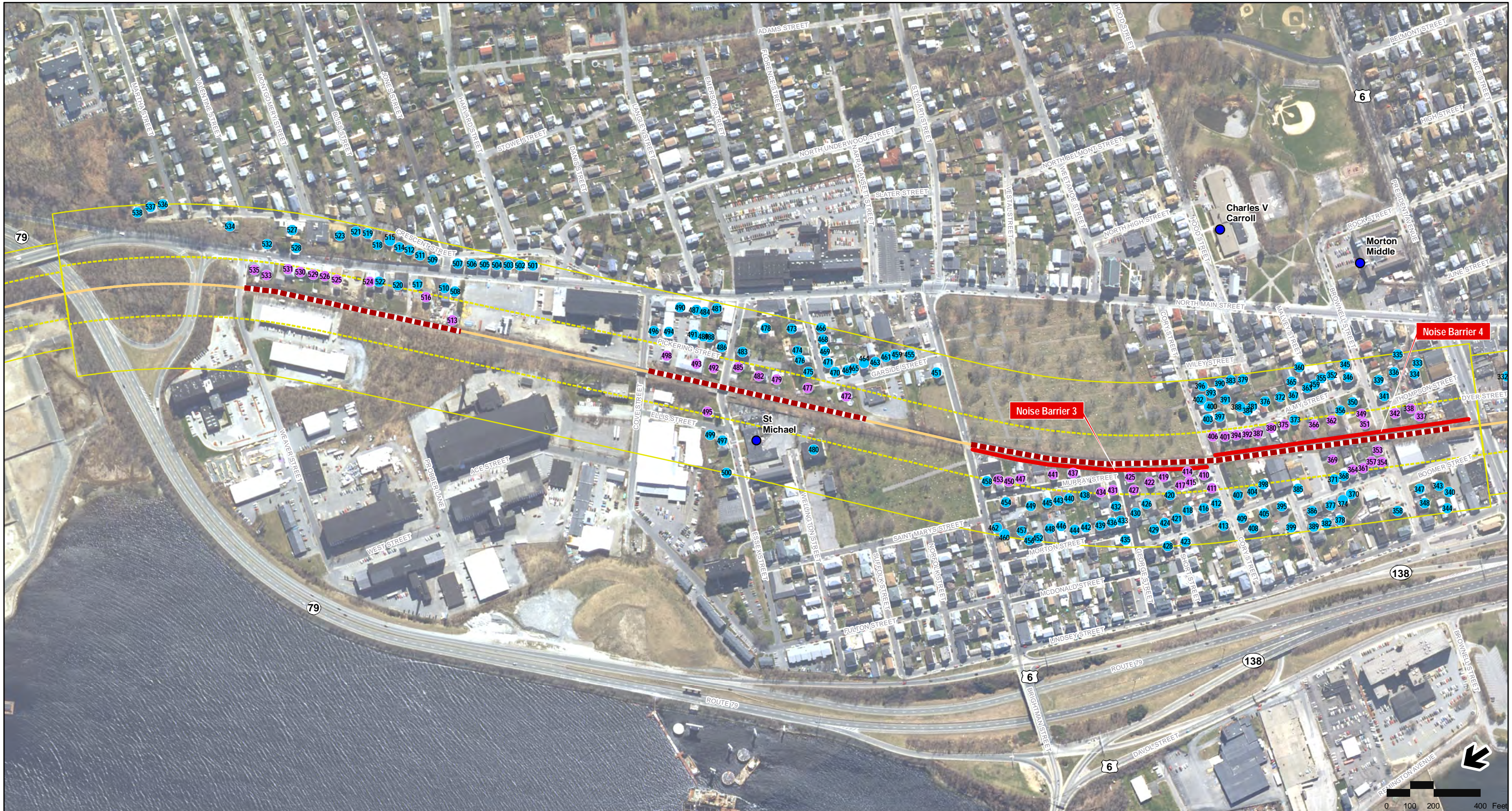
Figure 4.6-4g Stoughton/Whittenton Electric Alternative Noise Impacts and Mitigation and Vibration Mitigation Fall River Secondary (Detail)
