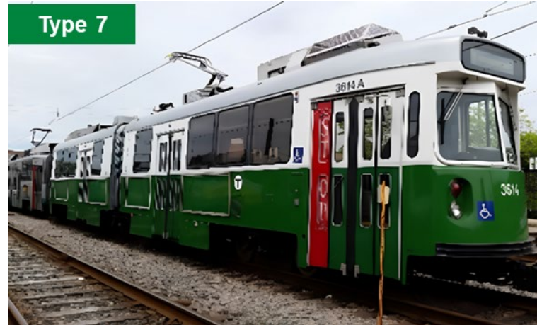
Type 7: Kinki Sharyo – Japan (1986-1988) Fleet: 103 Vehicles Age: 35+ Years Service Life: 30 Years Length: 74 Feet
