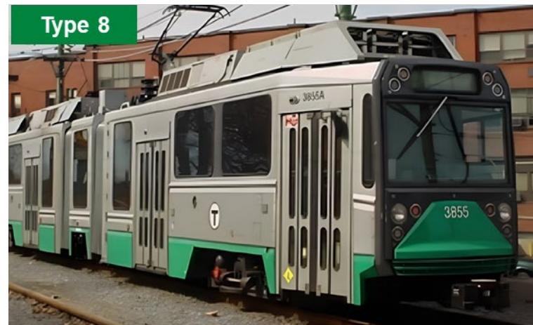
Type 8: Ansaldo/Breda – Italy (1999-2007) Fleet: 86 Vehicles Age: 17+ Years Service Life: 25 Years Length: 74 Feet
