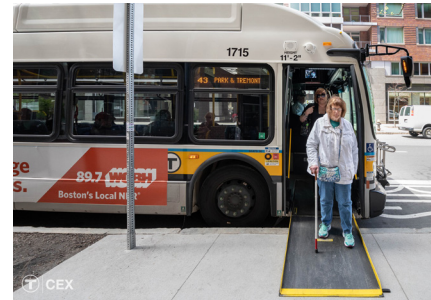
Downtown Boston bus stop with a paved, level, unobstructed path of travel and a fully deployed mechanical access ramp
