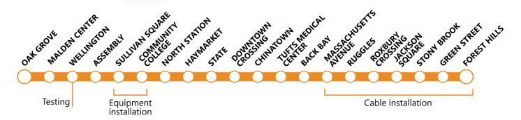
Orange Line Signals: Increasing capacity, through reducing headways with modernized signals
