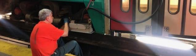
Today's Board action will provide services for the installation of the Green Line Train Protection System (GLTPS) carborne kits on the fleet of Green Line legacy vehicles. Outfitting the 103 Type 7's, 87 Type 8's & 24 Type 9's with newly designed safety equipment requires:
