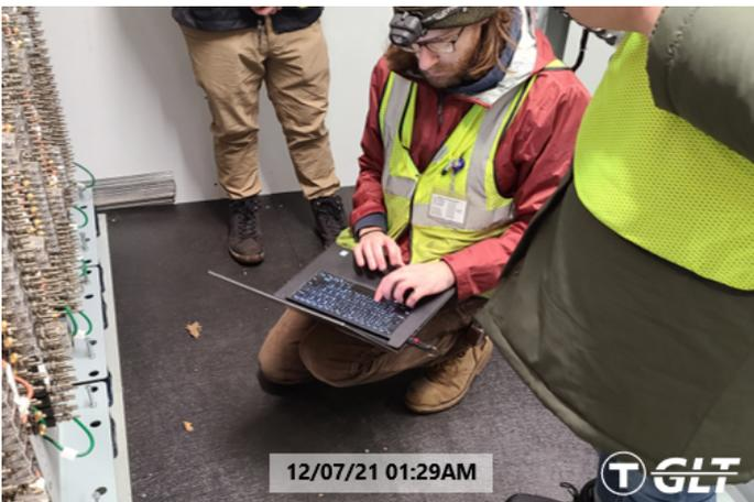
Timing Measurement of Signals (Fig. 5)
