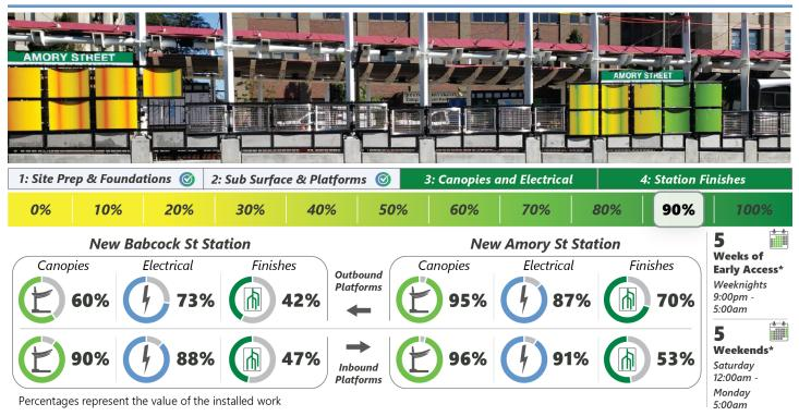
**<u>B Branch Station Consolidation Project</u>**: Consolidate four (4) existing Green Line stations on the B Branch along Commonwealth Avenue adjacent to Boston University, into two (2), fully accessible, brand new stations (Babcock & Amory).
