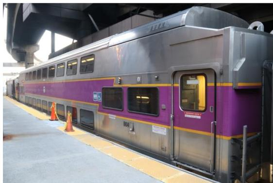
The MBTA's current bi-level trailer coach, pictured in **Figure F-8**, is used in all simulated locomotive-hauled consists. Its simulation parameters are shown in **Table F-9**. The trailer coach solely provides passenger accommodations and cannot be used as the lead unit on a train as it does not include a control cab.
