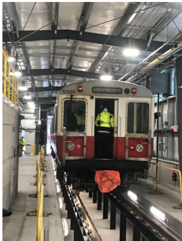
Completed a new Vehicle Testing Facility and Mobile Traction Power Substation providing static testing and maintenance capabilities for new vehicle testing and commissioning.
